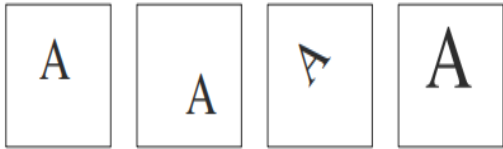
Figure 11.16 The identity of the object does not change when it is translated, rotated, or scaled. Note that this may not always be true, or may be true up to a point: 'b' and 'q' are rotated versions of each other. These are hints that can be incorporated into the learning process to make learning easier.
